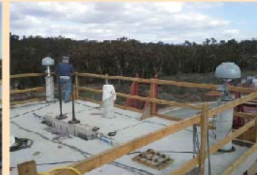
Rooftop NW GPS + MEMS accelerometer and collocated Episensor
