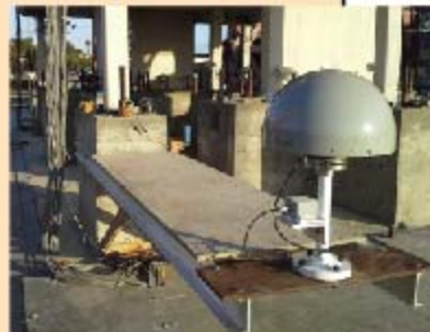
Foundation GPS + MEMS Accelerometer and Episensor
