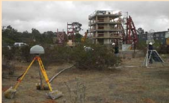
Foundation GPS + MEMS Accelerometer and Episensor
