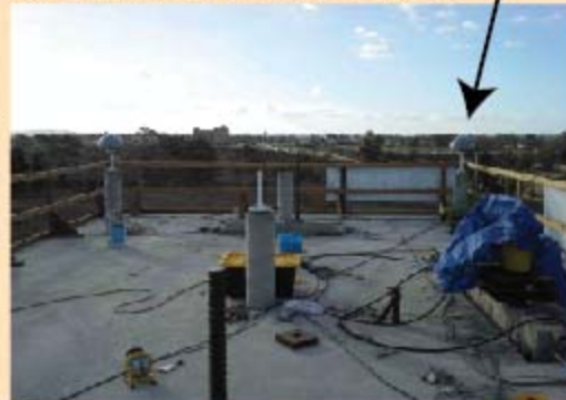
Rooftop NW GPS + MEMS accelerometer and collocated Episensor
